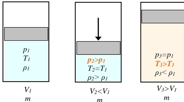
The system is absolutely leak proof, amount and mass of the filled medium is constant. To increase the pressure inside the cylinder the piston is pressed downwards ( $p_2 > p_1$ ), the gas is compressed, the density of the gas is increasing, the volume is decreasing. On the other hand, by heating the gas inside the cylinder ( $T_3 > T_1$ ), the density of the gas is decreasing and the volume is increasing!
