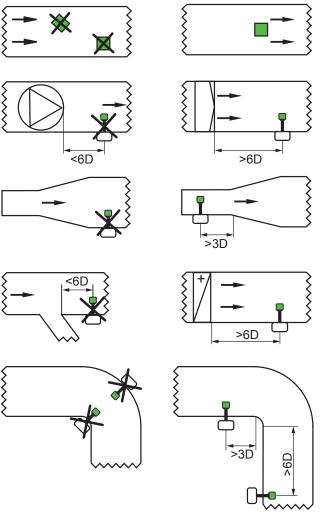
Install the sensor in the middle of the duct.
