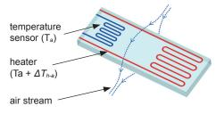
An E+E air velocity sensor consists of two resistors deposited on a thin glass substrate. One resistor is used as temperature (T) sensor and measures the temperature of the ambient air flowing along the sensor  $(T_a)$ .
