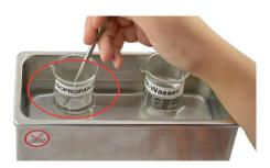
Fig. 1 Sensing head in isopropyl alcohol
