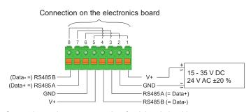
Connection assignment appropriate for daisy-chain wiring
