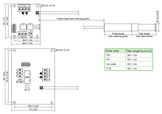
Fig. 1 Dimensions of EE1950
