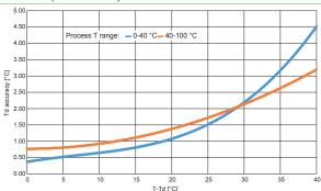
Accuracy of the calculated relative humidity (RH) out of the measured Td and the reading of an additional T sensor with ±0.2 °C (3.6 °F) uncertainty.
