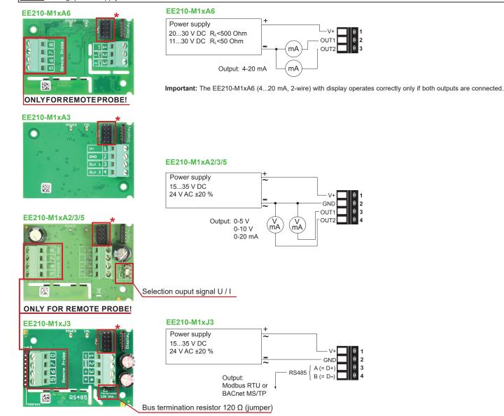
\* Configuration connector, see chapter SETUP AND ADJUSTMENT for detailed information
