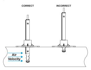
If the sensor probe is installed without a mounting flange make sure the air velocity sensor is aligned in parallel with the air stream.
