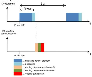
When the measuring time interval is > 15s, a measurement can be triggered by reading the status byte.
