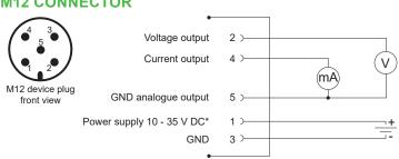
\*The supply circuit must be fused with ≤ 8A
