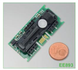
An optional kit facilitates easy configuration and adjustment of the module. The measurement interval can be set according to the application requirements; by this the average current consumption can be reduced to less than  $60 \mu A$  for battery-operated devices.
