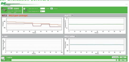
**Please note:** the relative humidity (RH) measurement is not implemented yet into the EE895 sensor module, the corresponding graph shows no curve and is headed by "n. def.".
