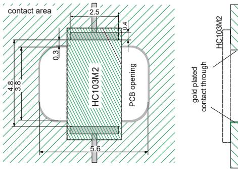
For shortest response time, in case of mounting onto a printed circuit board (PCB), HC103M2 shall be positioned over an opening to allow enough air circulation around the sensor.
